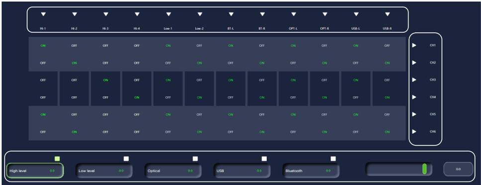
To configure signal routing, use the routing table, where all possible signal inputs are located horizontally, and all possible signal outputs are located vertically.
