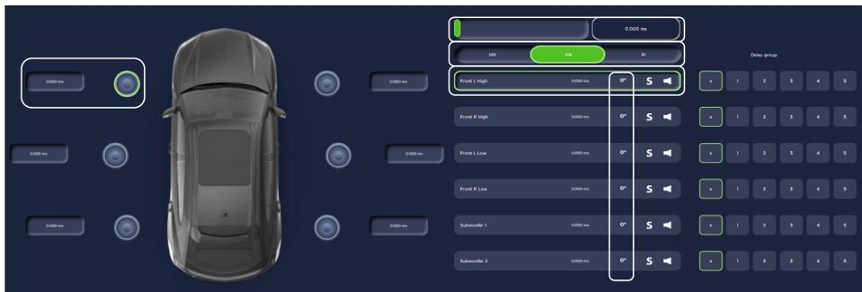
If you need to reverse the signal phase from 0° to 180° on the selected channel, use the PHASE button.
