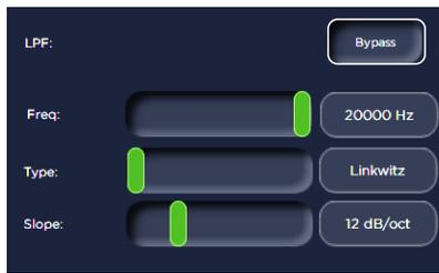
To temporarily disable the selected filter without resetting its settings, click the BYPASS button next to the filter name
